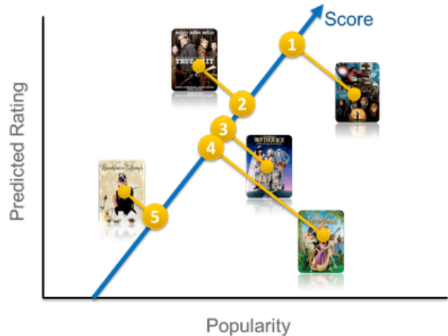
Figure 4: Constructing a basic personalized two-dimensional ranking function based on popularity and predicted rating
