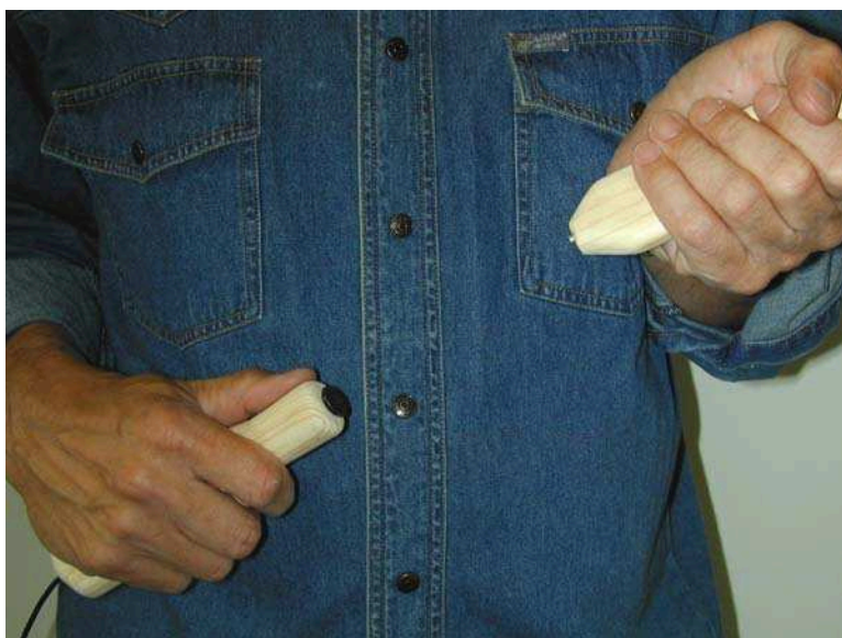
Figure 5.18: Control sticks for playing the VAG. Right-hand stick (on the left) includes an acceleration sensor as well as a small loudspeaker to send the distance measurement pulse. Left-hand stick (on the right) receives the pulse by an electret microphone.
