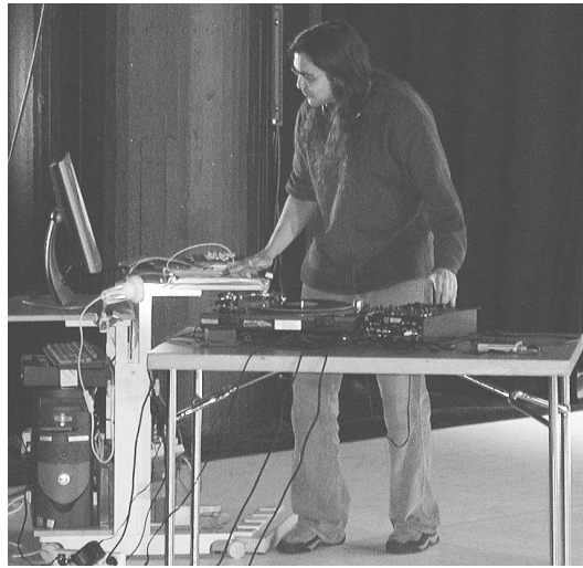
Figure 5.13: DJ 1210 Jazz scratching with Skipproof in a concert. The RadioBaton is operated with his right hand. Beside the computer screen is the lamp for the light sensor, on the floor is a rack of foot switches. His left hand is on the crossfader.
