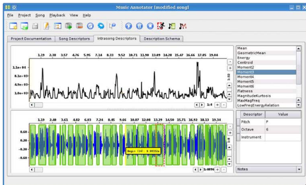
Fig. 10 Editing low-level descriptors and segments with the CLAM annotator. This tool provides ready-to-use descriptors such as chord extraction and can also be used to launch custom algorithms
