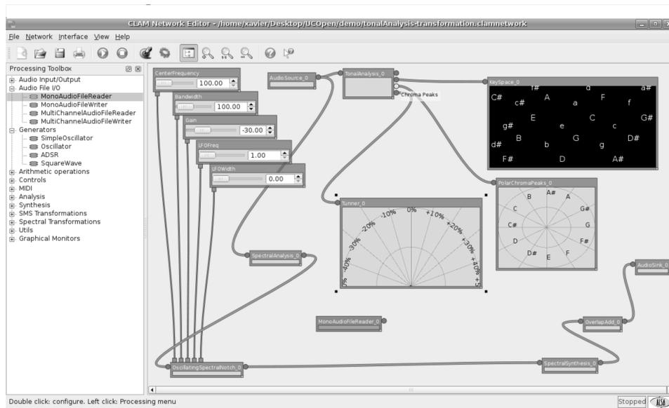
Fig. 4. NetworkEditor is the visual DSL for the CLAM framework. It can be used not only as an interactive multimedia dataflow application but also to build networks that can be run as stand-alone applications.
