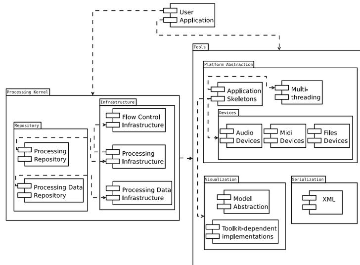
Fig. 2. CLAM Components. The CLAM framework is made up of a Processing Kernel and some Tools. The Processing Kernel includes an *infrastructure* that is responsible for the framework white-box behavior and *repositories* that offer the black-boxes. Tools are usually wrappers around pre-existing third party libraries. A user application can make use of any or all of these components.
