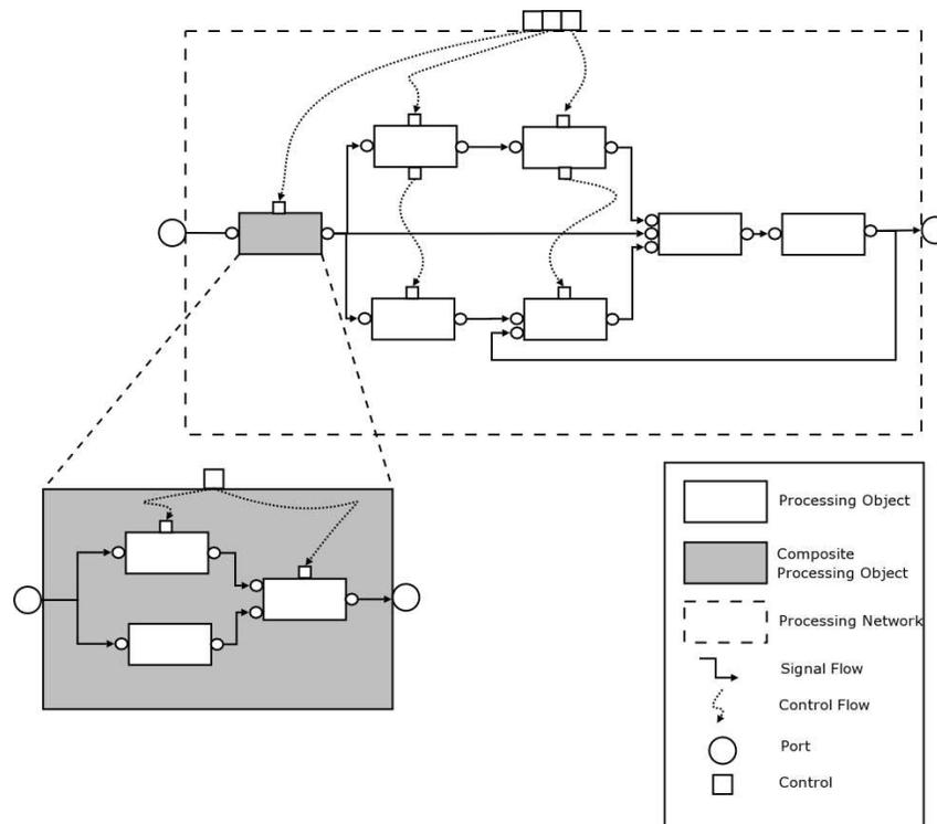
Fig. 3. Graphical model of a 4MPS processing network. Processing objects are connected through ports and controls. Horizontal left-to-right connections represents the synchronous signal flow while vertical top-to-bottom connections represent asynchronous control connections.
