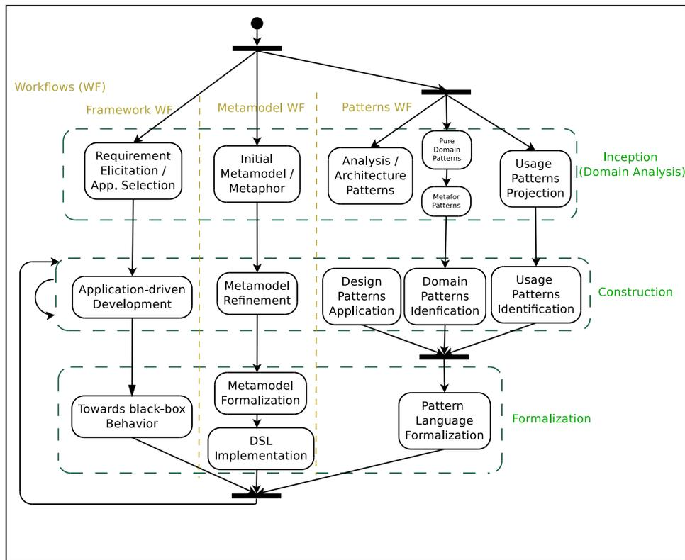
Fig. 1. Main activities in our framework development process model that includes three workflows – framework, metamodel, and patterns – and three phases – inception, construction, and formalization.
